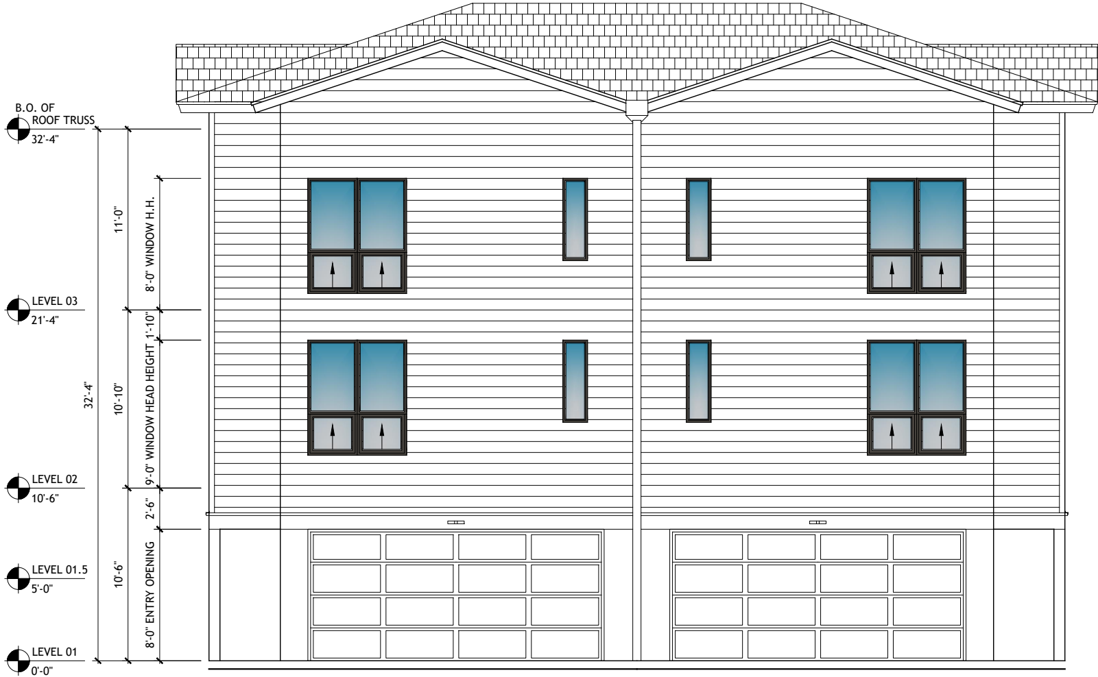
1 BUILDINGS 02, 05, & 06 GARAGE ELEVATION Scale: 1/8" = 1'-0"
