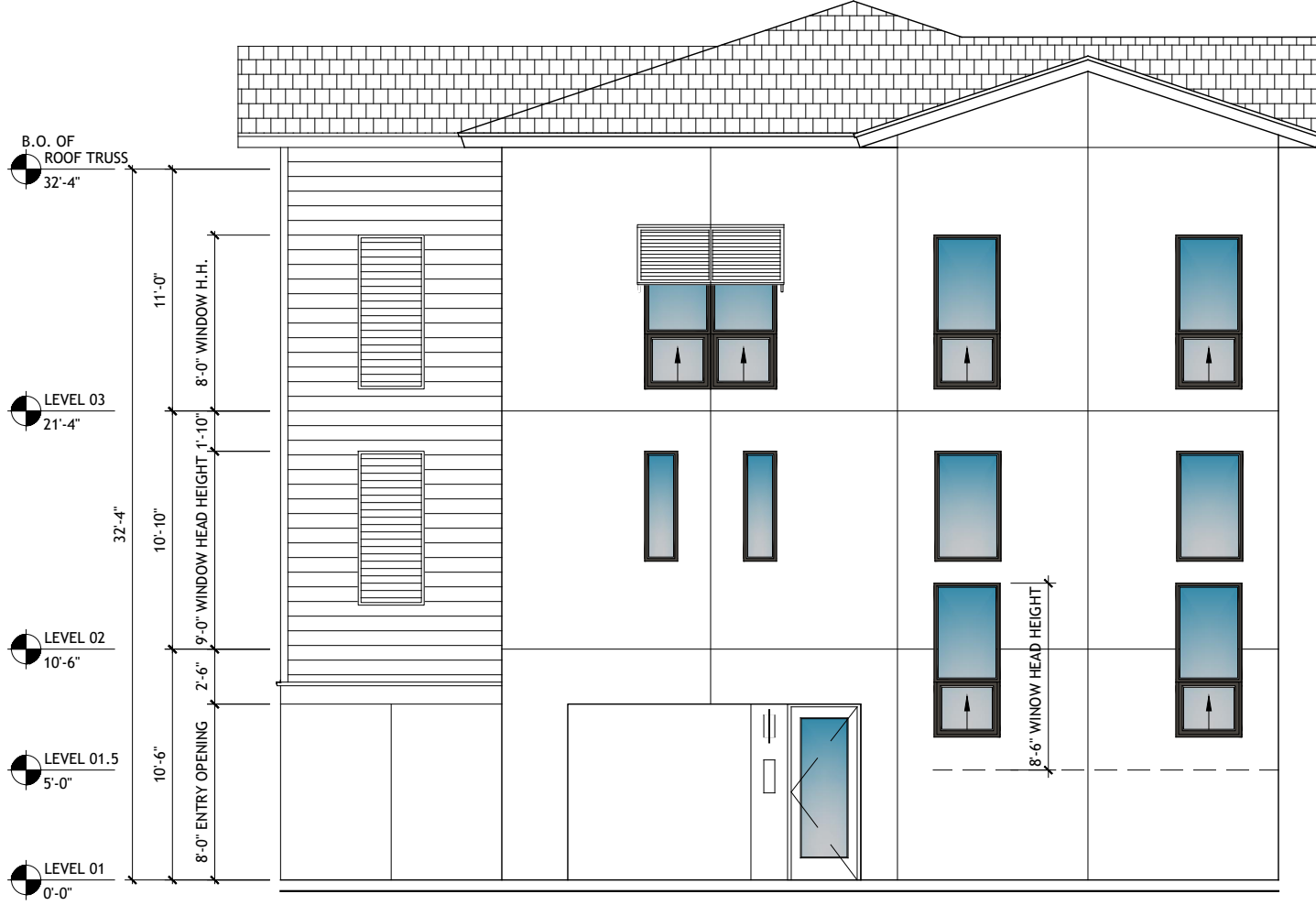
1 BUILDINGS 02, 05, & 06 SIDE ENTRY ELEVATION Scale: 1/8" = 1'-0"
