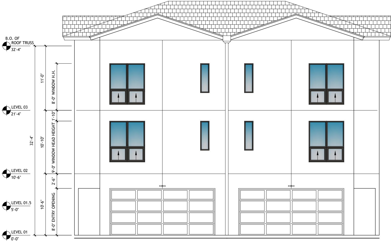
1 BUILDINGS 03 & 04 GARAGE ELEVATION Scale: 1/8" = 1'-0"
